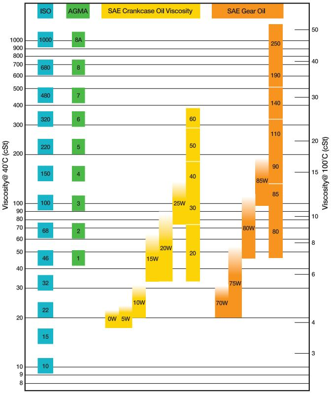
Winter grade (W) viscosities are also defined at low temperatures as well as minimum viscosities at 100°C (shown here). For a complete definition see the SAE J300 and J306 tables.
